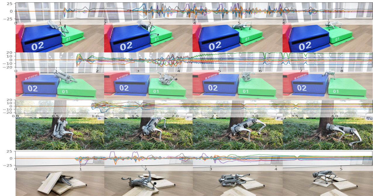
Fig. 2: Real-world experiments on challenging terrains (Flat, Foam, Stairs, Roots). Motor torques converge to similar values, indicating a near-optimal stable configuration.
