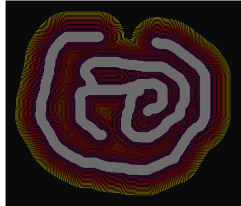
Fig. 1. Iso-contours of the SDF encoding Euclidean distance to obstacles.
