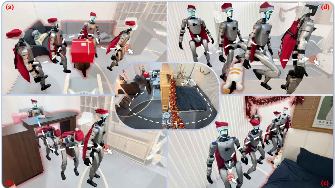
Fig. 1: Using a single generalist policy, our humanoid robot achieves collision-free traversal in cluttered indoor environments, including (a) detouring through narrow passages, (b) crouching under low-hanging obstacles, (c) squeezing through tight indoor spaces, and (d) hurdling over objects scattered on the floor.
